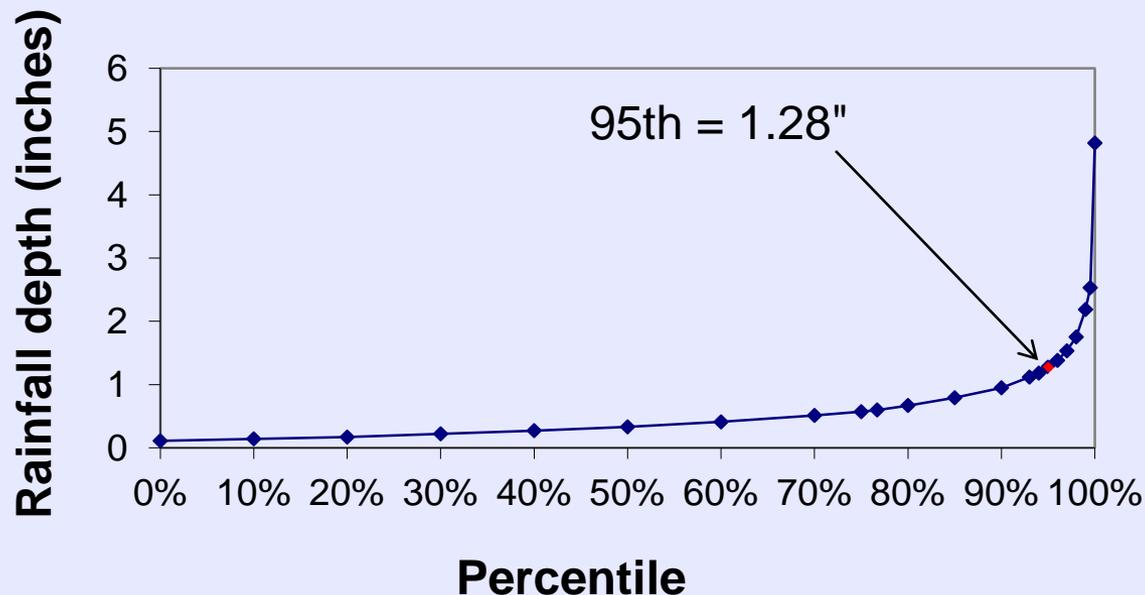
Volume of rain that would cover site footprint to a depth of the 95<sup>th</sup> percentile precipitation event (1.28 inches)
